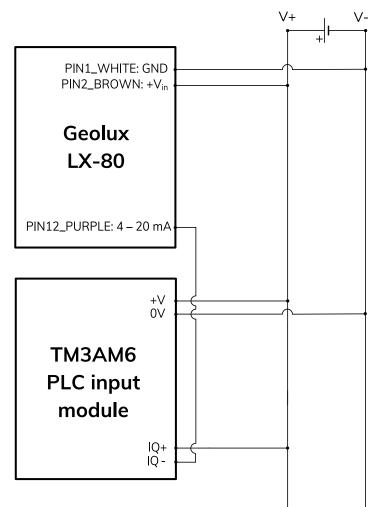
It is important to note that the 4 - 20 mA wire from the Geolux instrument should be connected to negative (-), not positive (+) terminal of the analog input port.
