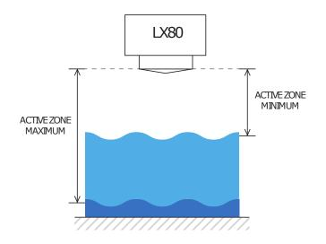
These parameters limits the operational range of the instrument. The instrument will detect water level only within the range set by the Active zone min. and Active zone max. parameters. These parameters is the best way to filter unwanted radar reflections from other structures and objects that are present on the monitoring site, that could cause false instrument readings.
