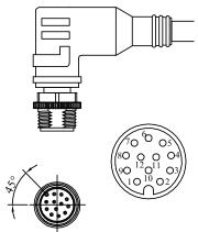
Picture 1. Level Meter Connectors
