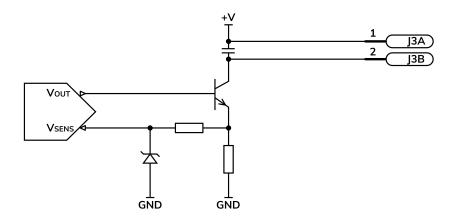
Picture 3. Analog 4 – 20 mA Output Internal Architecture
