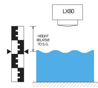
Setting the sensor height relative to the measurement is done using staff gauge. The sensor will output relative measurement of the actual water level based on its height above the riverbed.
