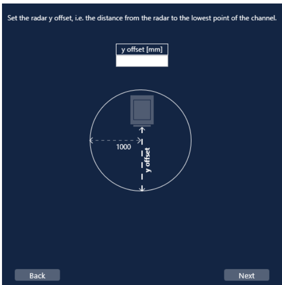
Picture 24. Defining the y Offset of the Radar
